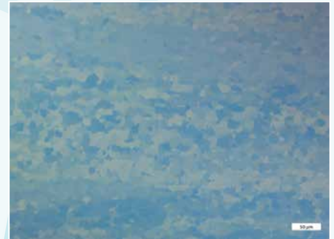
Titanio Puro, Grado 2, POL + Lambda Compensator, 200x
