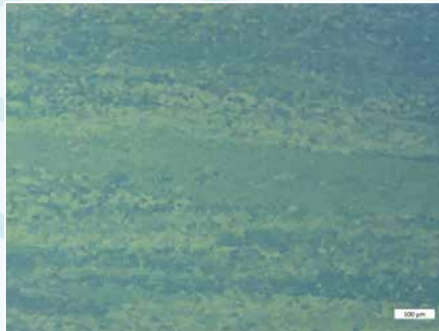
Titanio Puro, Grado 2, POL + Lambda Compensator, 100x
